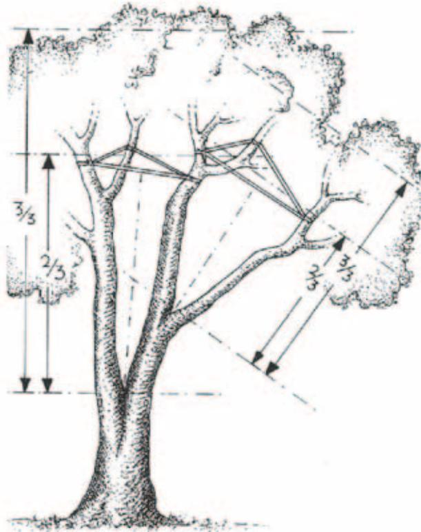
**Fig. 66.:** The height of installation for a single-level fracture prevention system (ZTV-Baumpflege 2006).
